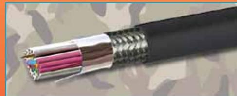
*Alpha's superior Supra-Shield® construction uses a three-layer aluminum/polyester/aluminum foil along with copper braid to offer exception shielding effectiveness over a wide range of frequencies.*
